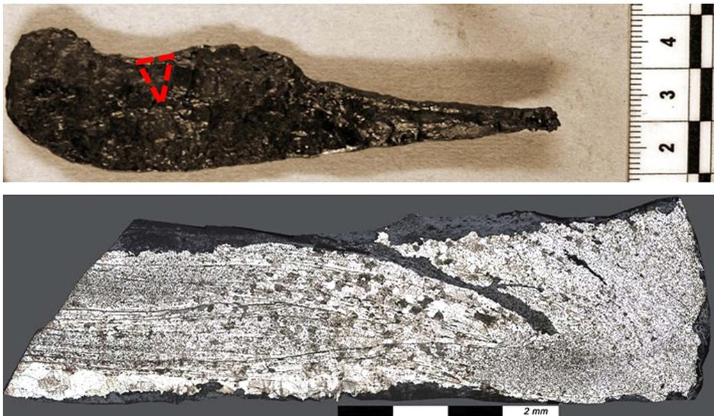
Figure 4. Unetched (top) and etched (bottom) section of scissors (OM, plain polarised light), showing a ferritic core, a steel edge and a line of slag inclusions between them (micrographs by David Larreina-Garcia).
