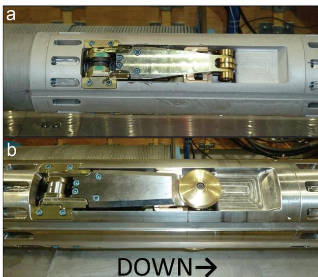
**Fig. 5.** The replicate coring system actuator sections showing the two styles of lever used for production drilling. (a) Anti-torque-style levers include sharp blades mounted on rollers. (b) Disk-style levers allow smooth movement in directions both vertical and tangent to the borehole wall.
