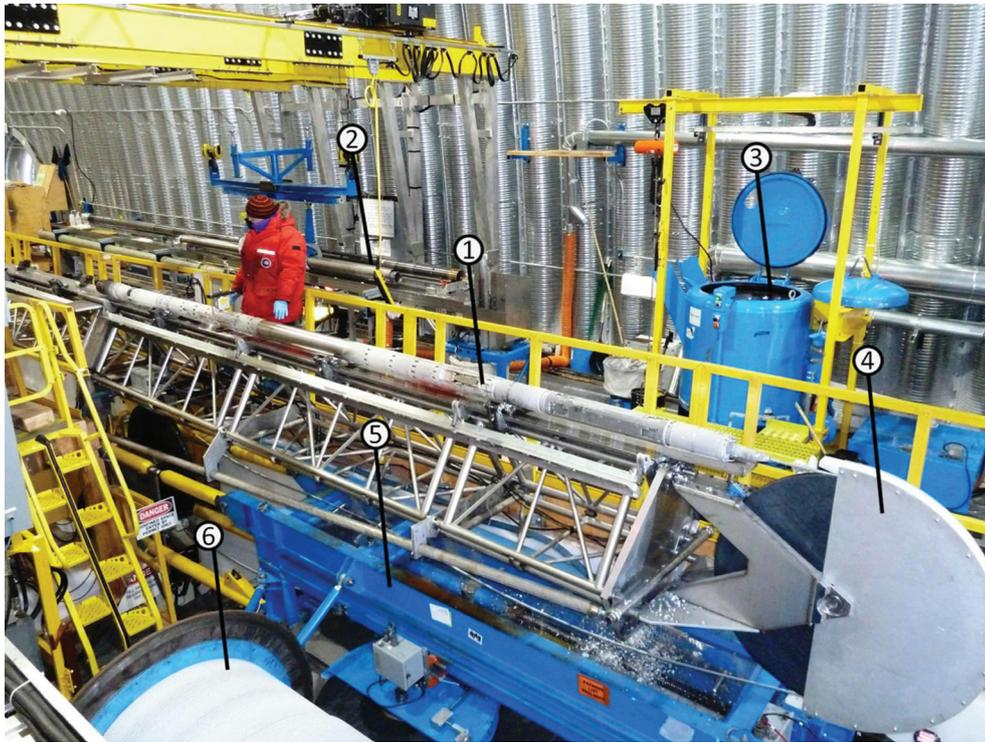
**Fig. 1.** The replicate coring system in the drilling arch at WAIS Divide: 1: downhole sonde (see also Figs 2 and 4); 2: ice-chip barrels at cleaning station; 3: centrifuge for removing drill fluid from ice chips; 4: crown sheave on tilting tower assembly; 5: cable level wind assembly; 6: 4000 m winch.
