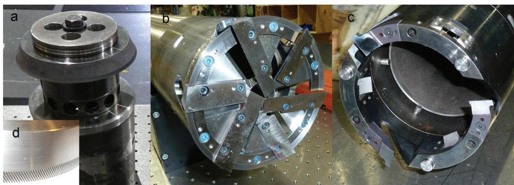
**Fig. 10.** The cutter heads used in production: broaching (a), milling (b) and coring (c). The inset (d) shows the critical serrated edge of the broaching cutter created by knurling the cutter before heat-treating. The white arrow in (b) identifies one of the six scoop cutters on the milling head.
