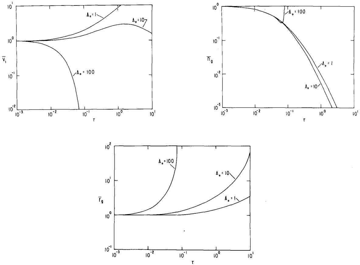
**Figure 1:** The variations of the normalized internal velocity, the number density and the grain radius with time, for different values of  $\Lambda_O$ , in the pure accretion model.
