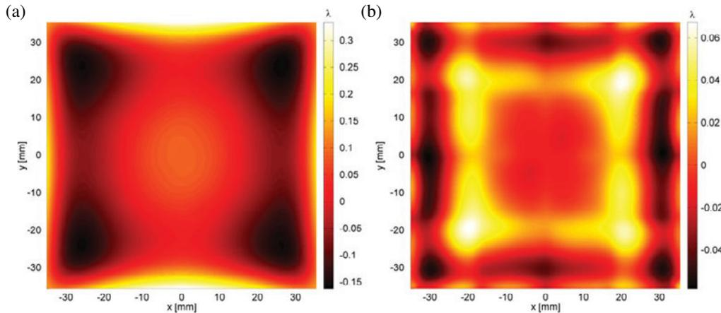
**Figure 13.** (a) Output OPD calculated in MIRÓ and shown in Figure 12(b) after subtraction of tilt and defocus. (b) Residual OPD after correction by the deformable mirror with 36 actuators.
