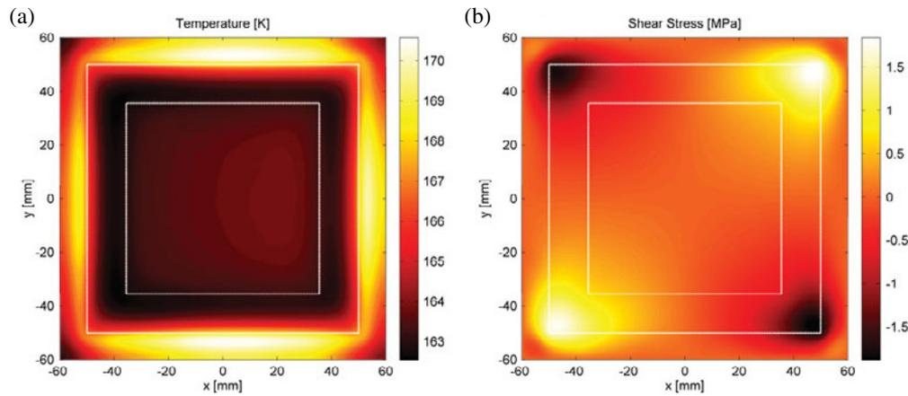
**Figure 10.** (a) Transverse distribution of temperature and (b) transverse distribution of the  $xy$  stress component in a longitudinal cut in the center of the laser slab.
