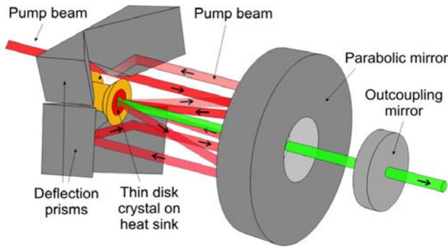
**Figure 1.** Schematic of the thin-disk cavity consisting of a parabolic mirror focusing the pump beam onto the thin-disk crystal. Multiple passes of the pump beam are made by means of deflection prisms. The cavity for laser beam extraction is formed by the thin-disk crystal and the outcoupling mirror.<sup>[14]</sup>
