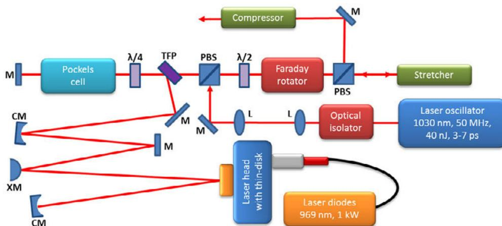
**Figure 3.** Schematic of the current status of Beamline B. Shown are flat mirrors (M), convex mirrors (XM), concave mirrors (CM), lenses (L), half and quarter waveplates ( $\lambda/2$ ,  $\lambda/4$ ), PBS, and a thin film polarization beam splitter (DP).
