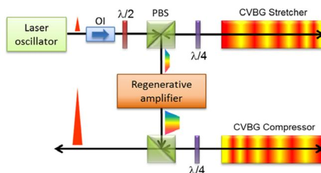
**Figure 4.** Schematic of the current status of Beamline C. Shown are an optical isolator (OI),  $\lambda/2$ ,  $\lambda/4$ , PBS, and a CVBG stretcher and compressor.
