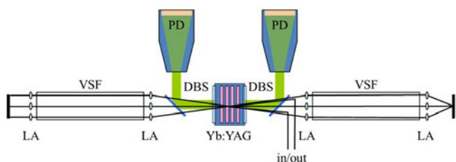
**Figure 6.** Schematic of the 10 J cryogenic multi-slab amplifier. It consists of  $\text{Yb}^{3+}$ :YAG ceramic slabs in the laser head (Yb:YAG), dichroic beam splitters (DBSs), lens arrays (LAs), vacuum spatial filters (VSFs), and homogenized pump diode laser modules (PDs).
