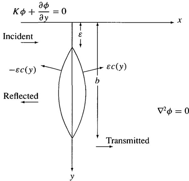
FIGURE 3. Symmetric slender barrier  $a < y < b$ .
