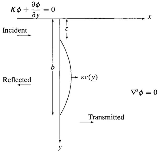
FIGURE 2. Nearly vertical plate  $a < y < b$ .
