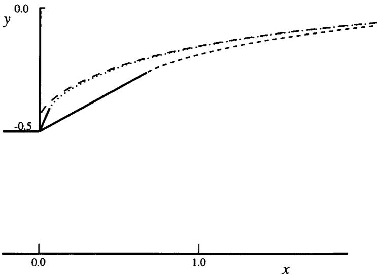
FIGURE 4. Free surface shapes computed for a fixed submergence depth at infinite Froude number, but with different bow slopes. The effect of the bow is local, with all free surfaces asymptoting to the same shape as  $x$  increases.
