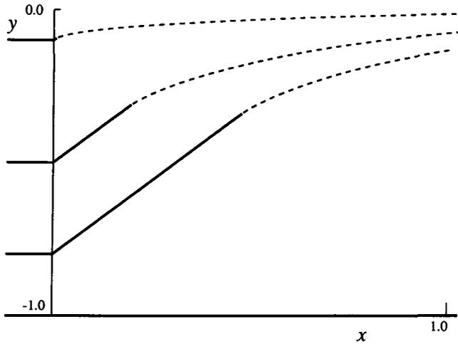
FIGURE 3. Some free surface shapes for a fixed bow slope with different submergence depths for the infinite Froude number case. All asymptote to the level  $y = 0$ , and the bottom of the channel is at  $y = -1$ . Solid lines depict the bow, dashed lines the free surface.
