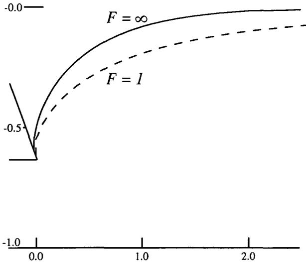
FIGURE 6. Free surface shapes for a bow which slopes backward for  $F = 1$  and  $F = \infty$ . Note that the separation is still smooth, but very close to the corner. The slope is  $126^\circ$  and  $D/H = 0.63$ .
