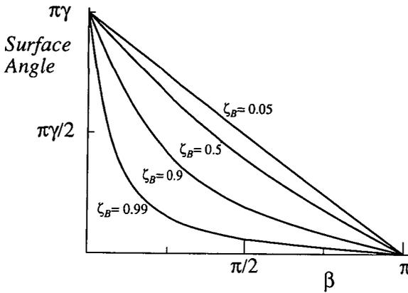
FIGURE 2. Diagram showing the angle of the free surface for several values of  $\zeta_B$ . The solutions are the same if scaled by the bow slope,  $\gamma$ .
