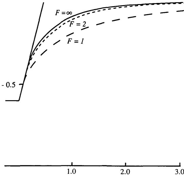
FIGURE 5. Comparison of free surface shapes for different values of the Froude number,  $F = \infty$ ,  $F = 2$ ,  $F = 1$ , where the slope is  $54^\circ$  and the draft  $D/H = 0.6$ .
