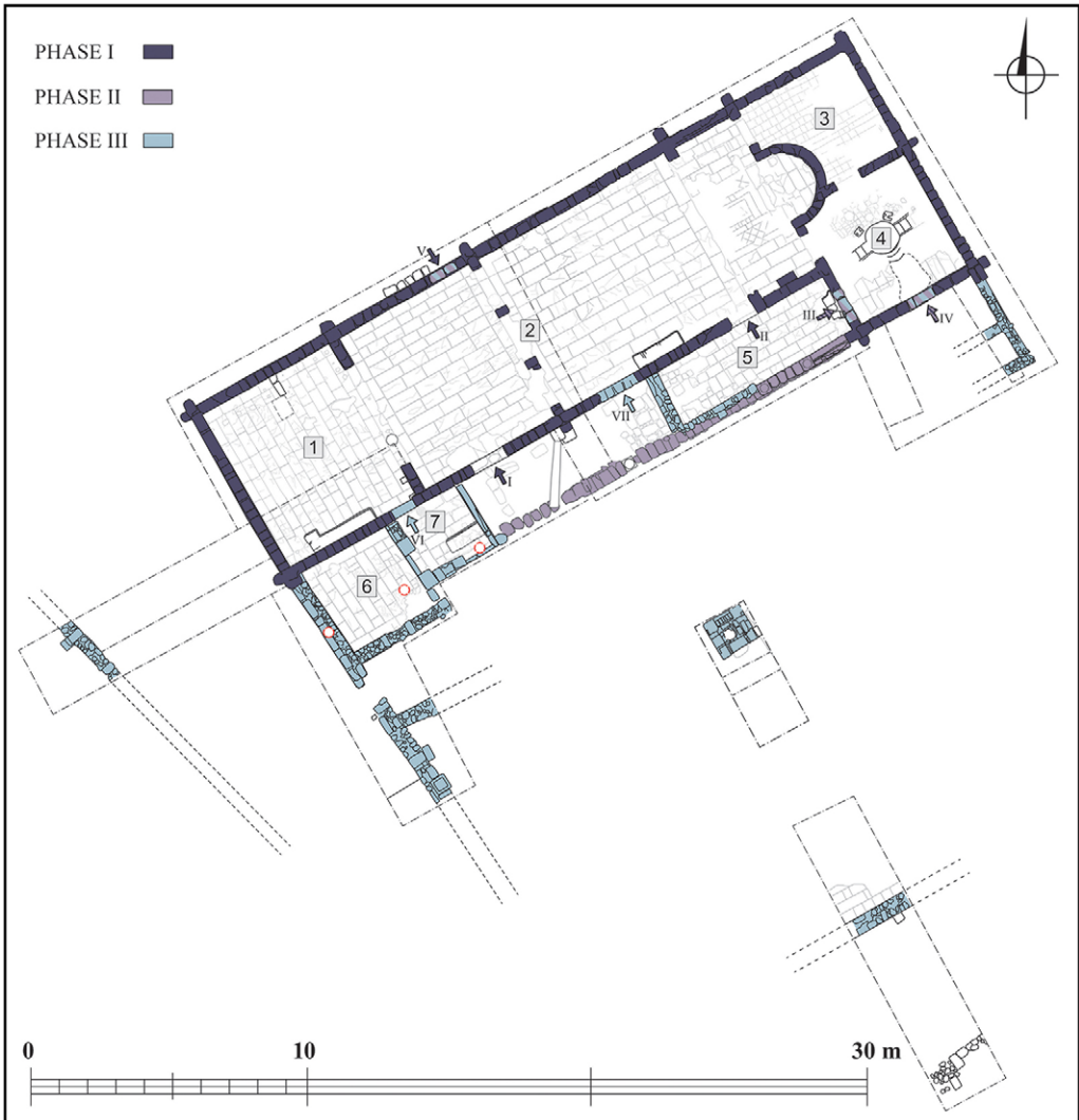
Figure 3. N1 plan with construction phases (figure by A.B. Kutiak & P. Zakrzewski).
