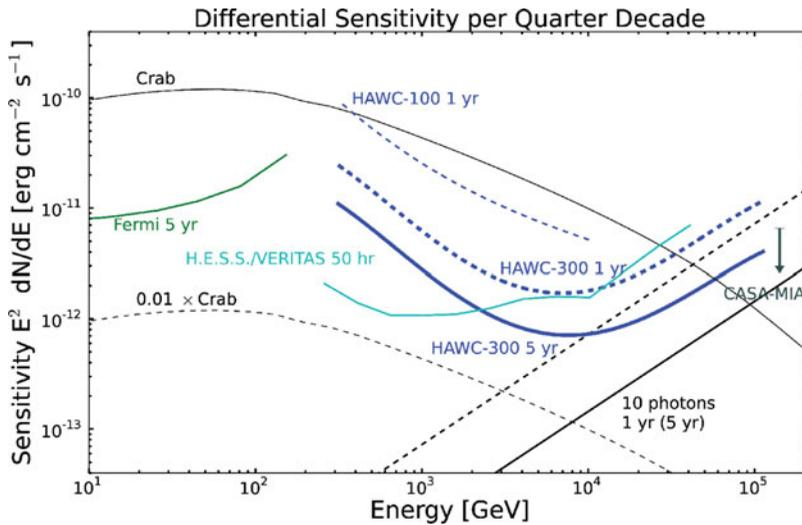
**Figure 2.** The differential sensitivity of HAWC to point sources.
