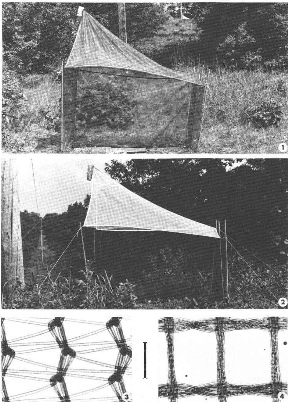
FIGS. 1-4. Malaise trap design, construction, and location: 1, fine mesh trap at bottom site (Note: pan traps installed beneath and second trap in the distance at top of rise); 2, coarse mesh trap at top site; 3,4, photomicrographs of mesh types, scale line 0.5 mm: 3, fine (warp direction, vertical); 4, coarse (warp direction, horizontal).
