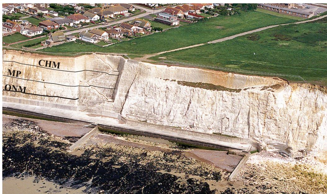
FIG. 13. Low-angle aerial photograph of the zig-zag steps cut into the cliff of Campanian chalk at Peacehaven, Sussex. The section between the Old Norse Marl (ONM) and the Castle Hill Marl (CHM) was sampled. Stratigraphy based on Mortimore (1986). MP is the Meeching Marl Pair.
