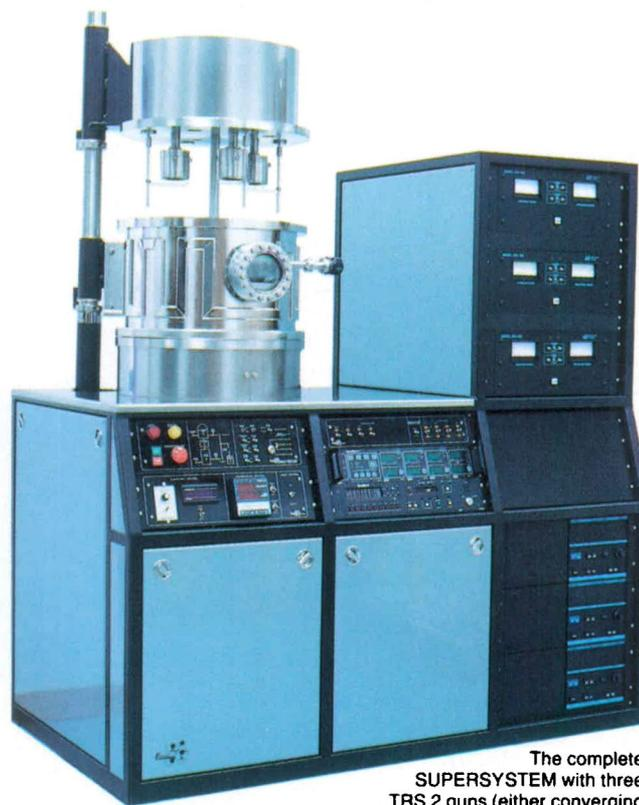
The complete SUPERSYSTEM with three TRS 2 guns (either converging or parallel) for Cu, Ba, Y oxide deposition
