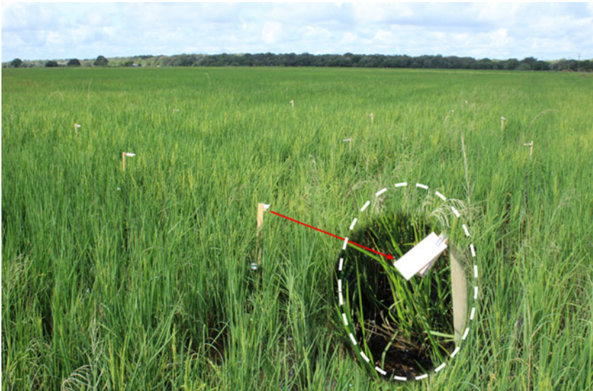
Figure 5. Placement of Kromekote cards on wooden poles in the experimental field for assessing spray droplet distribution. The inset is a close-up of the Kromekote card setup.
