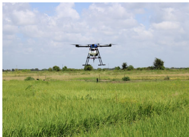
Figure 4. Remotely piloted aerial application system (Leading Edge® Precision Vision 35X; RPAAS) used in the study for targeting individual weed escapes/patches.
