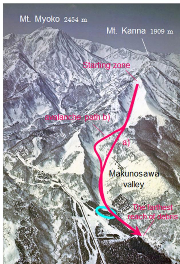
**Fig. 1.** Overview of Makunosawa valley. The two lines represent paths of the avalanche: (a) the straight route over the ridge; (b) the curved route along a stream. Part of the avalanche flowed into the cedar forest located in the ellipse.
