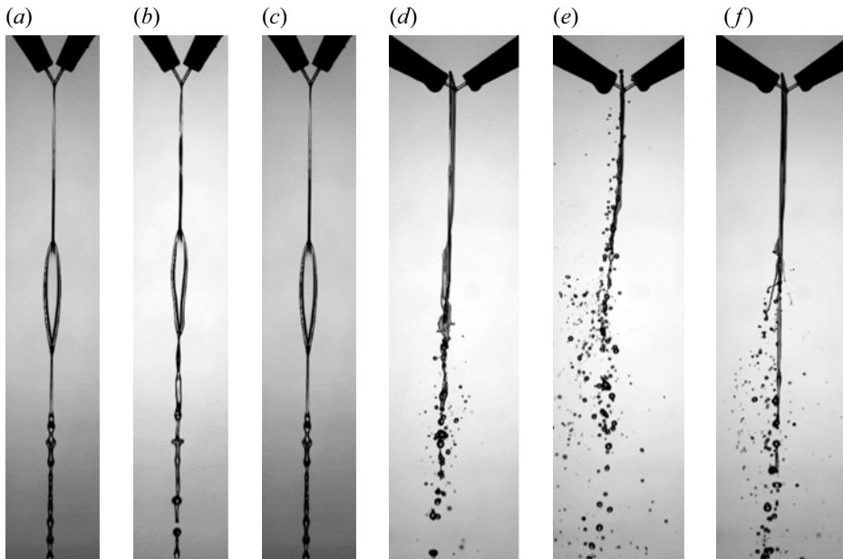
Figure 12. Observed side views of the sheet in the thinning region alone: (a–c)  $2\theta = 60^\circ$ ,  $We = 130$ , (a) unexcited case, (b,c) thinning region alone, (b)  $We = 130$ , 120 Hz and (c)  $We = 130$ , 200 Hz; (d–f)  $2\theta = 120^\circ$ ,  $We = 282$ , (d) unexcited case, (e,f) thinning region alone, (e)  $We = 282$ , 120 Hz and (f)  $We = 282$ , 200 Hz. Here SPL = 110 dB.
