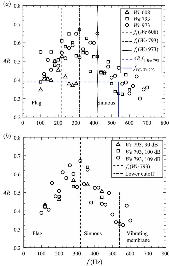
Figure 7. Effect of forcing frequency on the wave aspect ratio, for  $2\theta = 90^\circ$ . (a) Effect of Weber number on transition frequency. Here,  $f_i$  is the first forcing frequency (100 Hz) and  $f_{LC}$  is the lower cutoff frequency for  $We = 793$ . (b) Effect of SPL on transition frequency.
