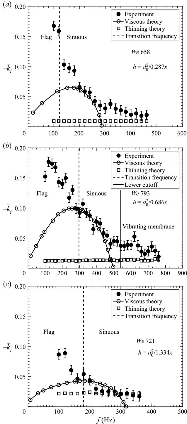
Figure 5. Comparison of the measured growth rates with the growth rate predicted by considering the viscous effects, for (a)  $2\theta = 60^\circ$ , (b)  $2\theta = 90^\circ$  and (c)  $2\theta = 120^\circ$ . The gas velocity profile in the viscous case is accounted for by using the modified Stokes model.
