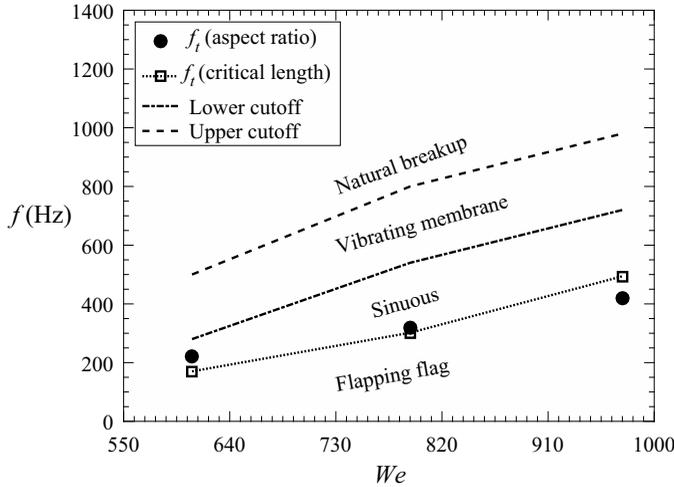
Figure 9. Transition frequencies separating the two instabilities as a function of Weber number.
