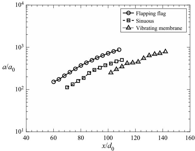
Figure 15. Spatial amplitude growth ( $2\theta = 60^\circ$ ,  $We = 658$ , 110 dB) for flapping flag (120 Hz), sinuous (260 Hz) and vibrating membrane type (460 Hz). Here  $a_0$  is the initial perturbation amplitude given by the acoustic source.
