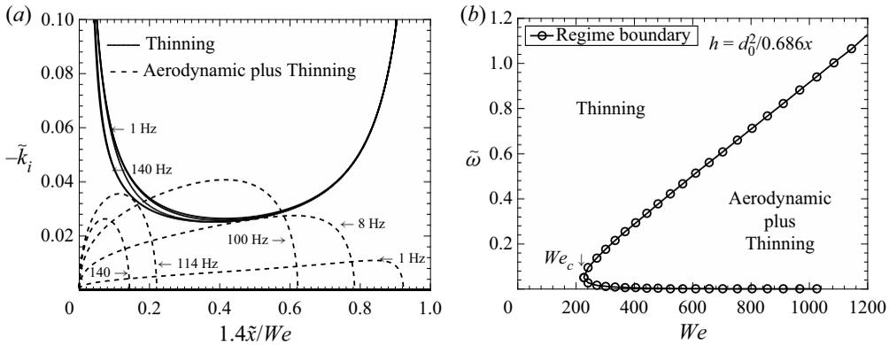
Figure 16. (a) Predicted growth rate by Squire's theory (aerodynamic) and thinning theory as a function of distance on the sheet axis for  $We = 302$ , and  $f = 1, 8, 25, 114$  and  $140$  Hz. (b) Regime map showing the dominance of either thinning or aerodynamic plus thinning effect. The dotted line separates the two regimes.
