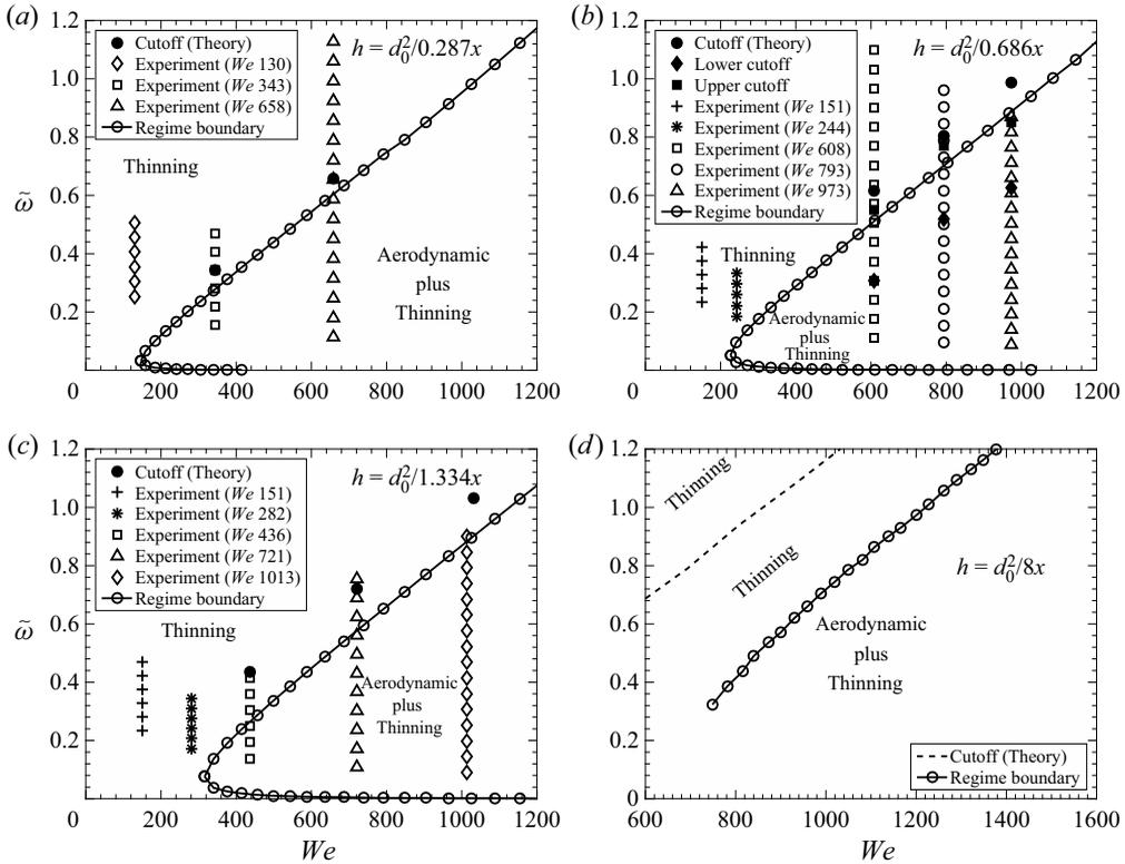
Figure 10. Regime maps showing the dominance of either the thinning effect or the aerodynamic plus thinning effect, for (a)  $2\theta = 60^\circ$ , (b)  $2\theta = 90^\circ$  and (c)  $2\theta = 120^\circ$ . The curve with circular markers separates the two regimes. (d) The cutoff frequencies using Squire's theory for a single jet impinging on a solid surface ( $h = d_0^2/8x$ ) (Bremond *et al.* 2007) and the upper boundary of the envelope for a similar configuration (Paramati *et al.* 2015).
