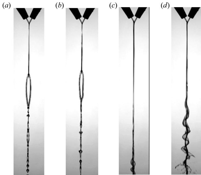
Figure 11. Sheet excitation at the same frequency ( $\omega = 0.3$ ) but for different Weber numbers: (a,b)  $2\theta = 60^\circ$ ,  $We = 130$ , (a) unexcited case ( $\omega = 0$ ) and (b)  $\omega = 0.3$ , thinning region; (c,d)  $2\theta = 60^\circ$ ,  $We = 658$ , (c) unexcited case ( $\omega = 0$ ) and (d)  $\omega = 0.3$ , aerodynamic plus thinning region. Here SPL = 110 dB.
