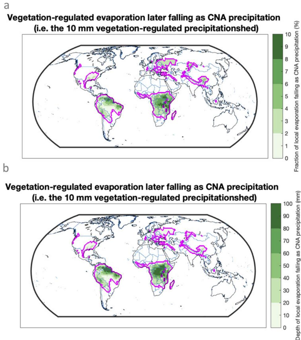
**Figure 4.** Global distribution of regions that provide vegetation-regulated evaporation to downwind CNA regions, as a fraction of total evaporation that falls as precipitation (a) and in total  $\text{mm yr}^{-1}$  of water (b). The pink outlines enclose the regions that provide  $10 \text{ mm yr}^{-1}$  or more of annual evaporation to global CNA regions.
