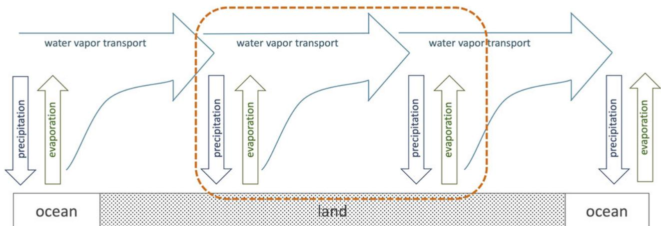
**Figure 1.** Schematic representation of atmospheric branch of water cycle, emphasizing moisture recycling that occurs over land. Within the orange dashed box, precipitation that is primarily of oceanic origin falls onto land, and the water that evaporates is from the land surface. This water is transported through the atmosphere, falls out as precipitation again, and is then re-evaporated on land again. Used with permission from Keys (2016).
