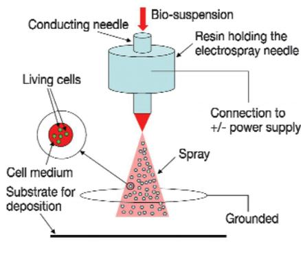
Figure 1. Schematic of the electrohydrodynamic jetting equipment.
