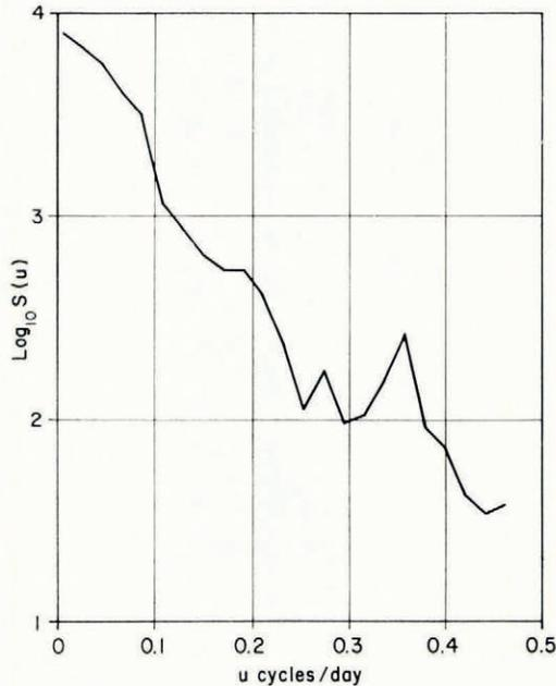
Fig. 7. Estimates of the power spectrum of Þjórsá at Urriðafoss.
