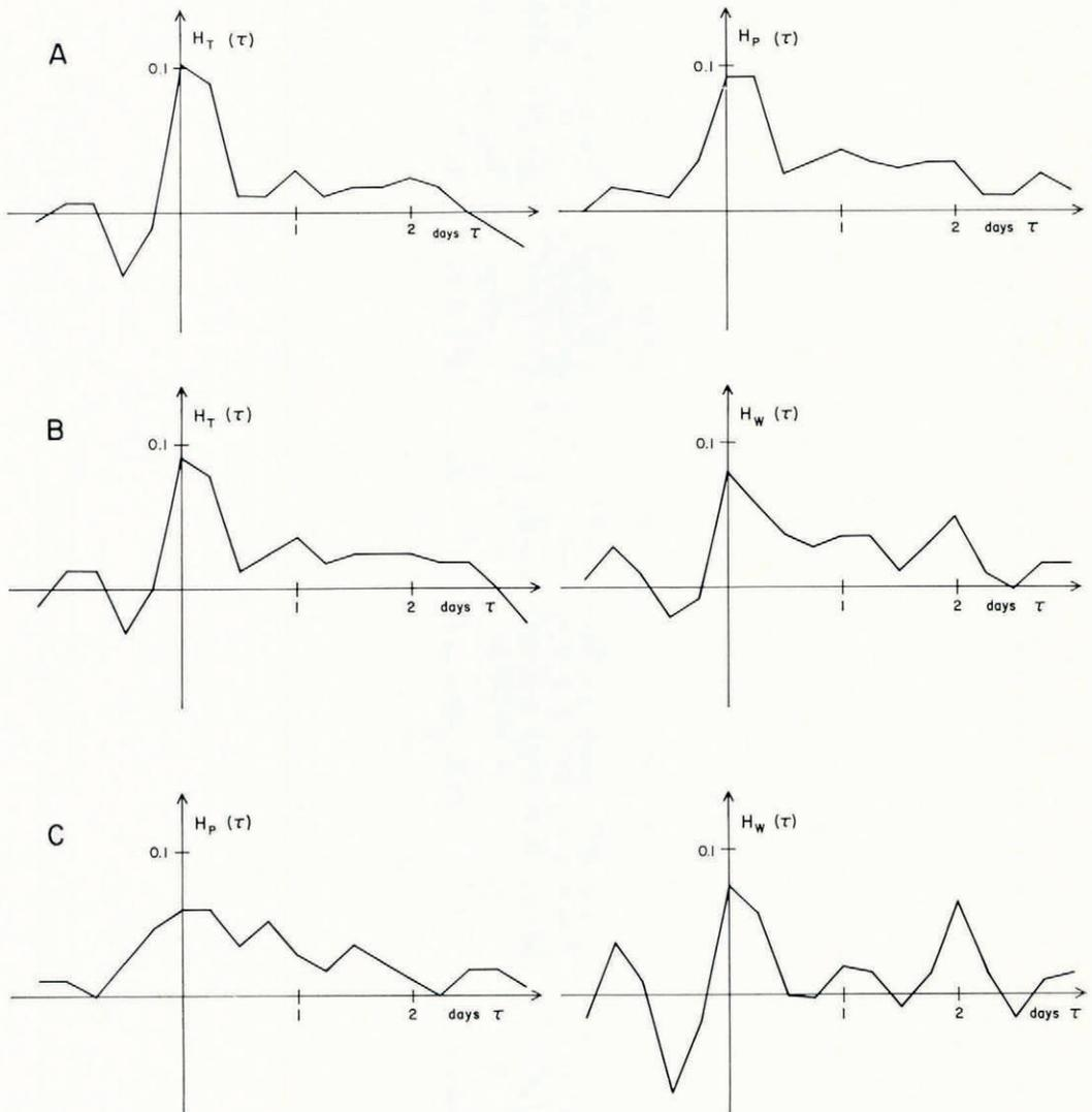
Fig. 9. Estimates of the impulse response of Tungná to meteorological variables. In A, the independent variables are temperature and precipitation, in B temperature and wind, and in C precipitation and wind.
