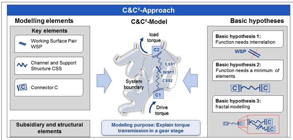
Figure 2: C&C<sup>2</sup>-approach and its elements according to Matthiesen et al. (2018)
