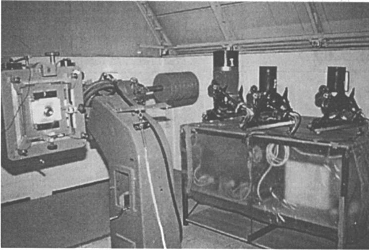
Figure 1. ASAS-3 in the 10" astrograph dome. From the left: 10" astrograph,  $F = 750\text{ mm}$  telescope, 2 wide-field instruments with 200/2.8 telephoto lenses.
