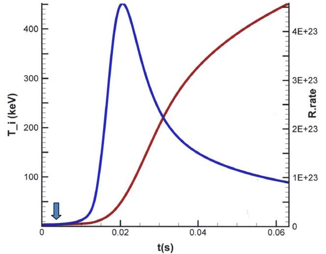
Figure 4. Temporal evolution of the reaction rate, and plasma ion temperature. The blue arrow indicates the end of operation of the  $\mu$ CF in the spark fusion part of the device which correspond to 1  $\mu$ s.
