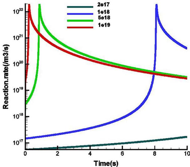
**Figure 5.** Temporal evolution of the reaction rate. The curves correspond to different initial values of the alpha particles produced by the  $\mu$ CF in the spark part of the device: (a) red  $10^{19} \text{ m}^{-3}$ , green  $5 \times 10^{18} \text{ m}^{-3}$ , blue  $10^{18} \text{ m}^{-3}$  and deep green  $2 \times 10^{17} \text{ m}^{-3}$ .
