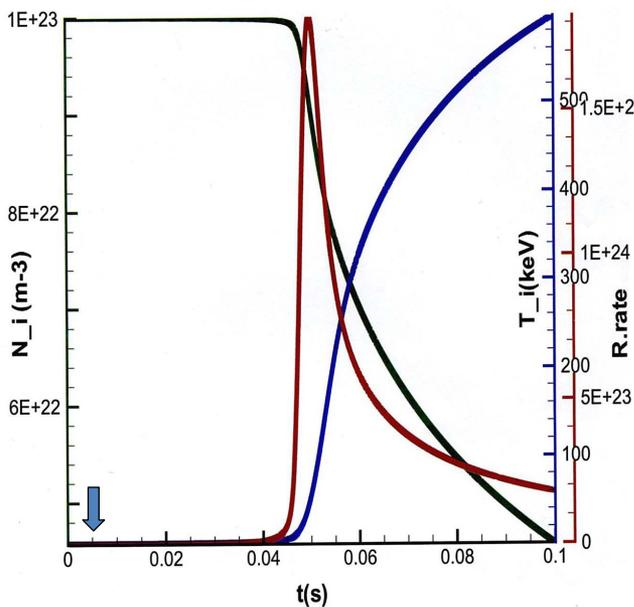
Figure 3. Temporal evolution of the reaction rate, plasma ion density and plasma ion temperature. The blue arrow indicates the end of operation of the  $\mu$ CF in the spark fusion part of the device which correspond to 1  $\mu$ s.
