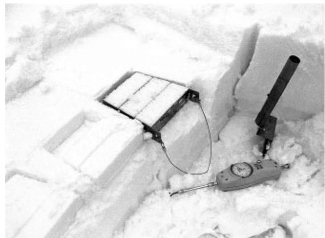
Fig. 1. Shear frame tester with an area of  $0.025 \text{ m}^2$ .
