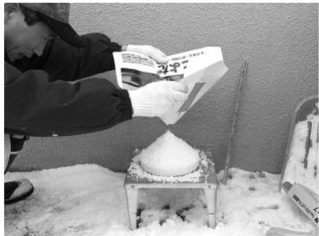
Fig. 3. Measurement of the angle of repose.
