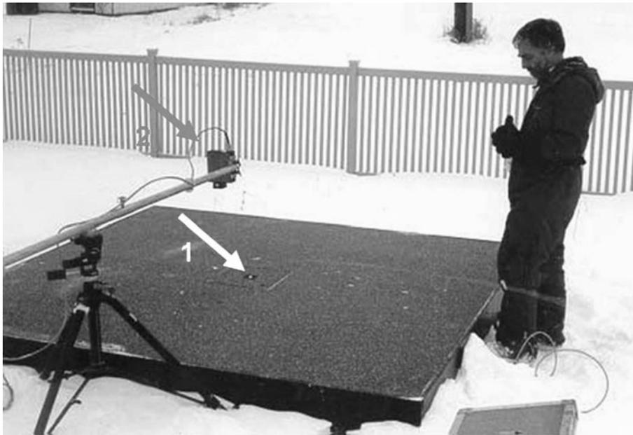
**Fig. 1.** The experimental set-up consisted of a 2.4 m × 2.4 m black plywood base with a detector mounted in the center (arrow 1) that measured transmitted irradiance. Incident and reflected irradiance were measured using a second detector that was mounted on a tripod (arrow 2).
