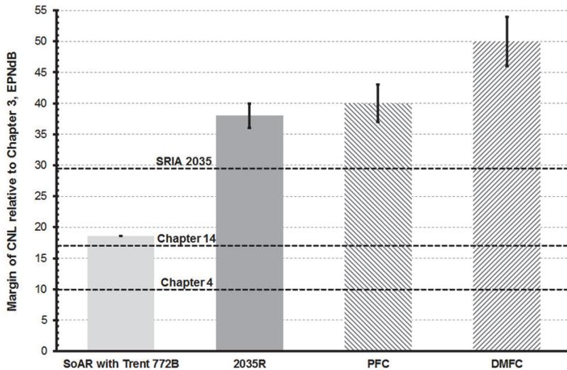
Figure 31. Results of external noise assessments for SoAR, 2035R, DMFC and PFC aircraft based upon CIAM-TsAGI in-house CNPP predictions.
