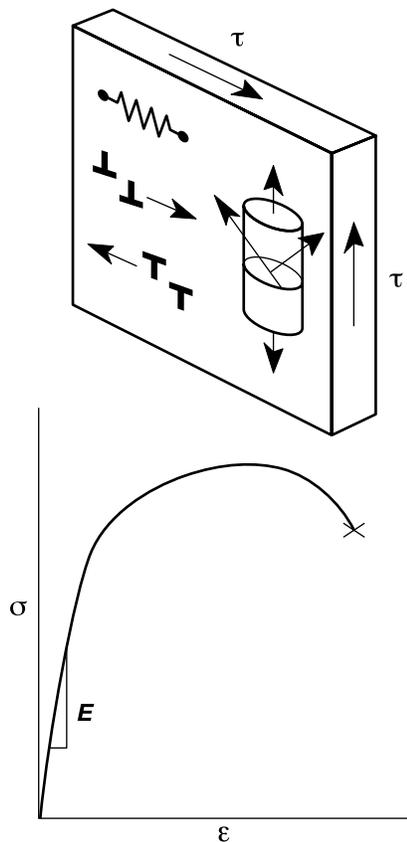
Figure 1. Graphical representation of an introductory-level treatment of the mechanical properties of materials. The graphic is designed to summarize and organize a significant amount of information covered in part of a course.  $\tau$  is shear stress,  $\sigma$  is normal stress,  $\epsilon$  is strain, and  $E$  is Young's Modulus.
