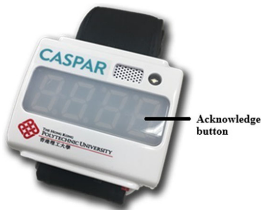
Figure 1. Wristwatch device with an acknowledge button that lights up and vibrates to remind the user to move the hemiparetic upper extremity.
