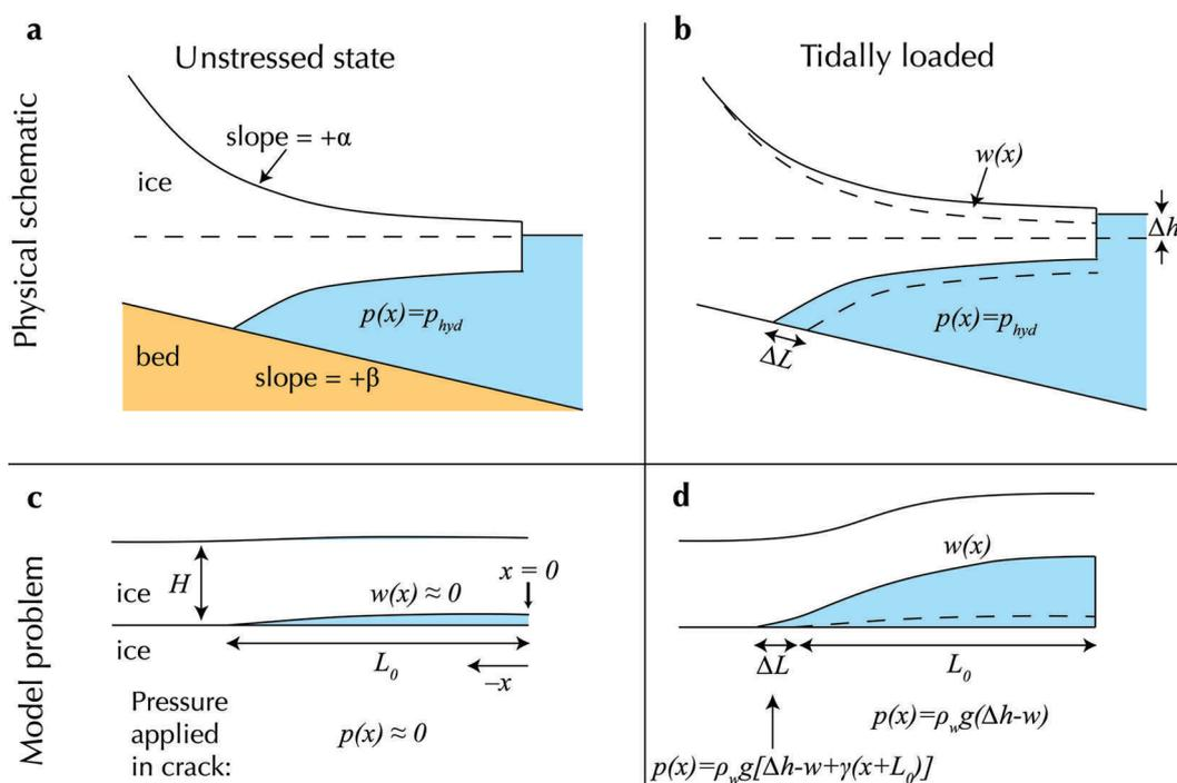
**Fig. 1.** (a, b) Schematic geometry under (a) unstressed and (b) tidally loaded cases. Water pressure,  $p$ , is assumed hydrostatic,  $p(x) = p_{hyd}$ , and both surface slope and bed slope are assumed constant near the grounding line. (c, d) Modeled crack-opening problem corresponding to the (c) unstressed and (d) tidally loaded cases.
