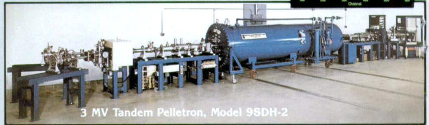
3 MV Tandem Pelletron, Model 9SDH-2
