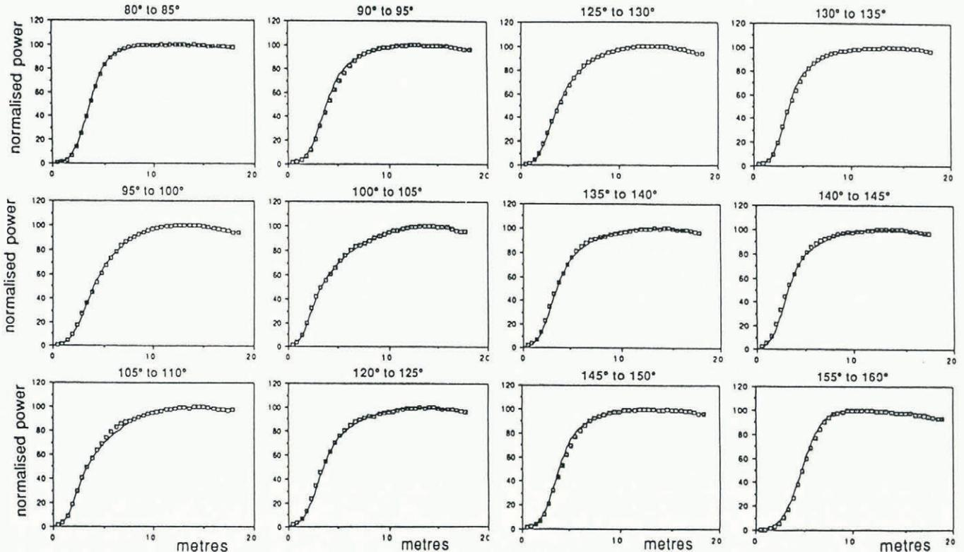
Fig. 8. Averaged wave forms from 5° longitude parts of Wilkes Land (squares), together with model ice-sheet wave-form fits (lines). The units of the horizontal axis are tens of centimetres. The plots are normalized to 100 in the vertical direction.
