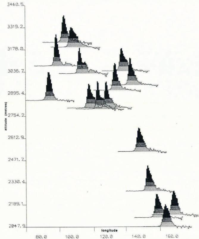
Fig. 9. Differentiated mean wave forms from  $5^{\circ}$  longitude parts of Wilkes Land at lat.  $72^{\circ}\text{S.}$ , shown located with mean altitude (metres: vertical axis) and longitude (the front of each histogram is referenced to longitude). The secondary peaks in the averaged differentials are not fitted by the model and may indicate the presence of sub-surface layers in the snow.
