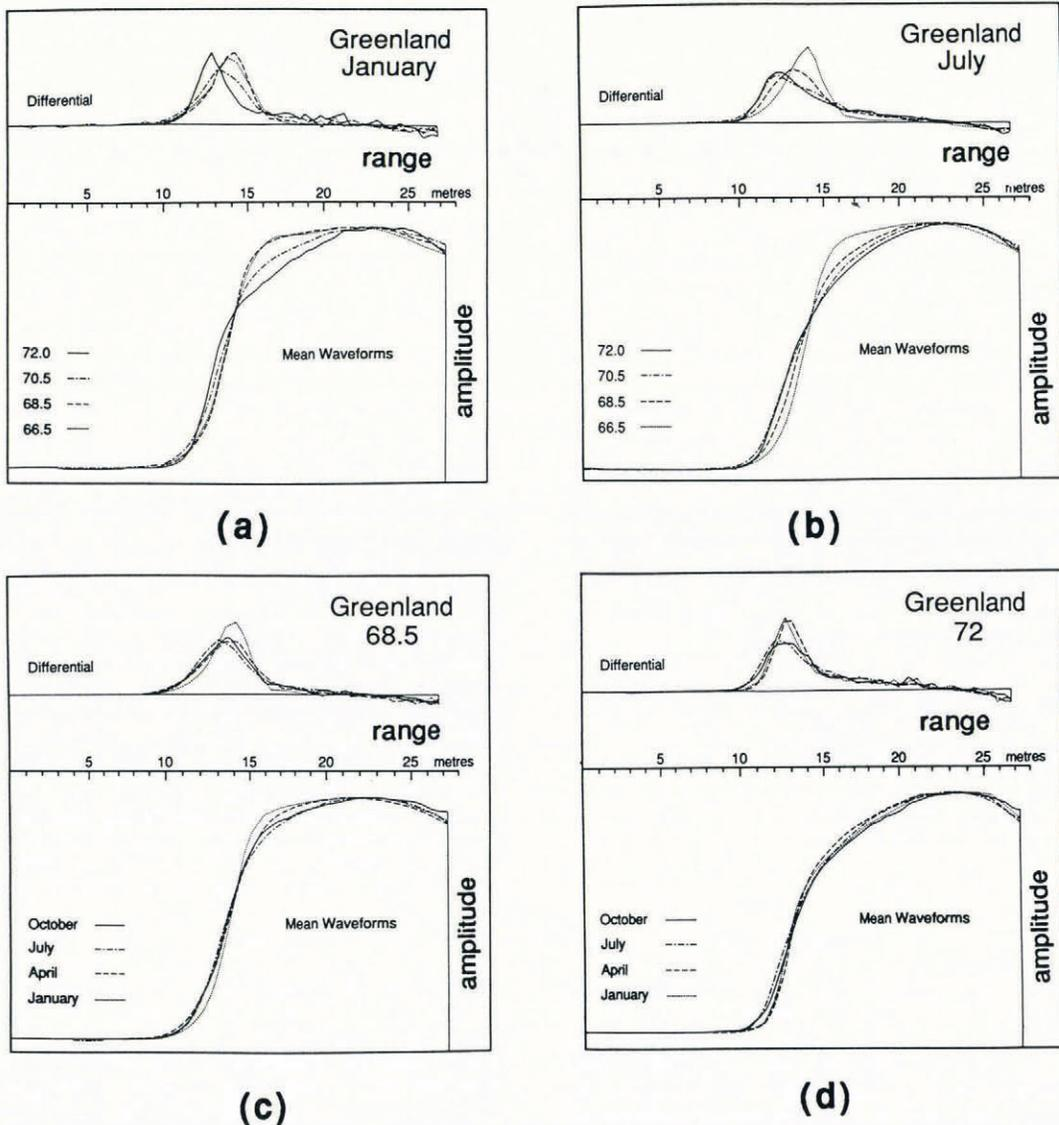
Fig. 5. Averaged Greenland ice-sheet return and differentiated mean return (the former normalized in the vertical direction). Averaged wave forms are all normalized in the vertical direction. Note the increased influence of volume scattering towards the north of the ice sheet (a) and (b).
