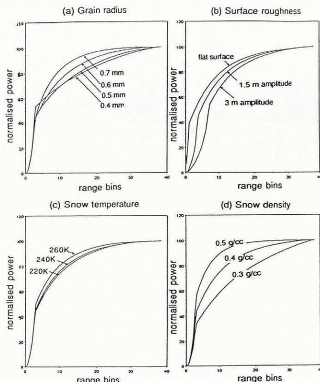
Fig. 1. Result of varying snow parameters on the shape of the radar return. The horizontal axes represent range bins and the vertical axes represent normalized signal amplitude (from Ridley and Partington, 1988). Note the similar effects of grain radius, snow density, and temperature on the shape of the return and the unique effect of surface roughness.
