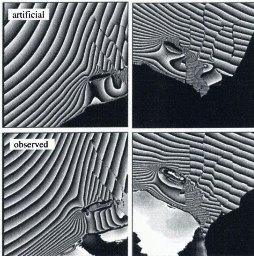
Fig. 5. The most favorable HIR experiment results and observed interferograms (from MacAyeal and others, *in press*, figs 6 and 7). In this experiment, a 50% coastal boundary-layer softening is applied and rifts are assumed to contain a 10 m thickness of melange ice. Image arrangement is as in Figure 4.
