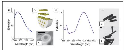
Extinction spectra of gold nanotubes that are 55 ± 7 nm in diameter and aligned in an AAO template (a). Cartoon depiction (b) and SEM image of aligned nanotubes (c). Extinction spectra of gold nanotubes suspended in  $D_2O$  (length = 258  $\pm$  42 nm; width = 55 ± 7 nm) (d), accompanied by their TEM (e, f) images. Scale bars are 100 nm. Reproduced with permission from Chem. Mater. 24 (6) (2012), DOI: 10.1021/cm203184d; p. 963. ©2012 American Chemical Society.
