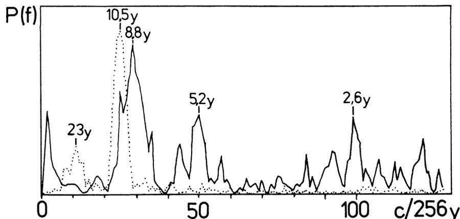
Fig 2. Power spectra from the  $\Delta^{14}\text{C}$  record (solid line) and sunspot record (dotted line). In order to avoid side lobes due to the length of the record, the spectra have been obtained by computing the amplitude of the sine wave best fitted to the data reduced to the first interval.
