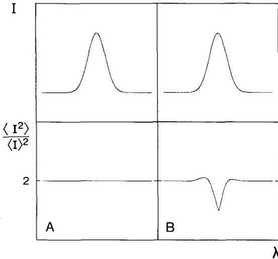
Fig.1. Hypothetical observation of two spectral features A and B that are indistinguishable by classical methods measuring intensity  $I$  vs. wavelength (top), reveal differences in photon statistics when observed with a quantum-optical spectrometer (bottom).
