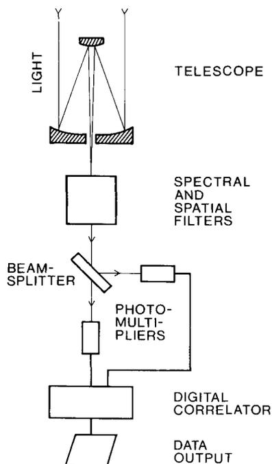
Fig.2. Possible configuration of a quantum-optical spectrometer, designed to measure intensity fluctuations in photon gas arriving from astronomical sources. The telescope collects light and selects the spatial feature to be observed, while the filter selects the desired spectral feature and defines the first-order coherence of light. Effects of correlated detector noise are minimized by the use of two photomultipliers whose output pulse trains are correlated in a digital processor.
