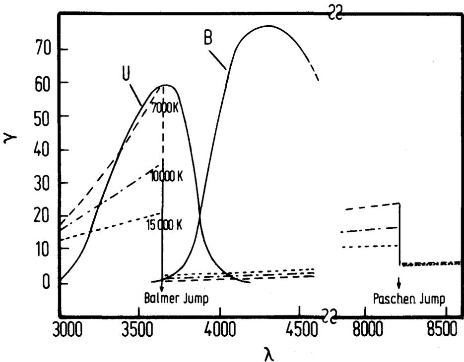
Fig. 4: Schematic picture of the temperature dependency of the Paschen- and Balmer emission coefficient (from Anderson and Kuhi, 1968) together with the sensitivity functions of U and B of the photoelectric UB<sub>V</sub> system (from Matthews and Sandage, 1963). The units of  $\gamma$  are  $10^{14} \text{ cm}^{-2} \text{ sec}^{-1}$ ;  $\lambda$  is in Angströms.
