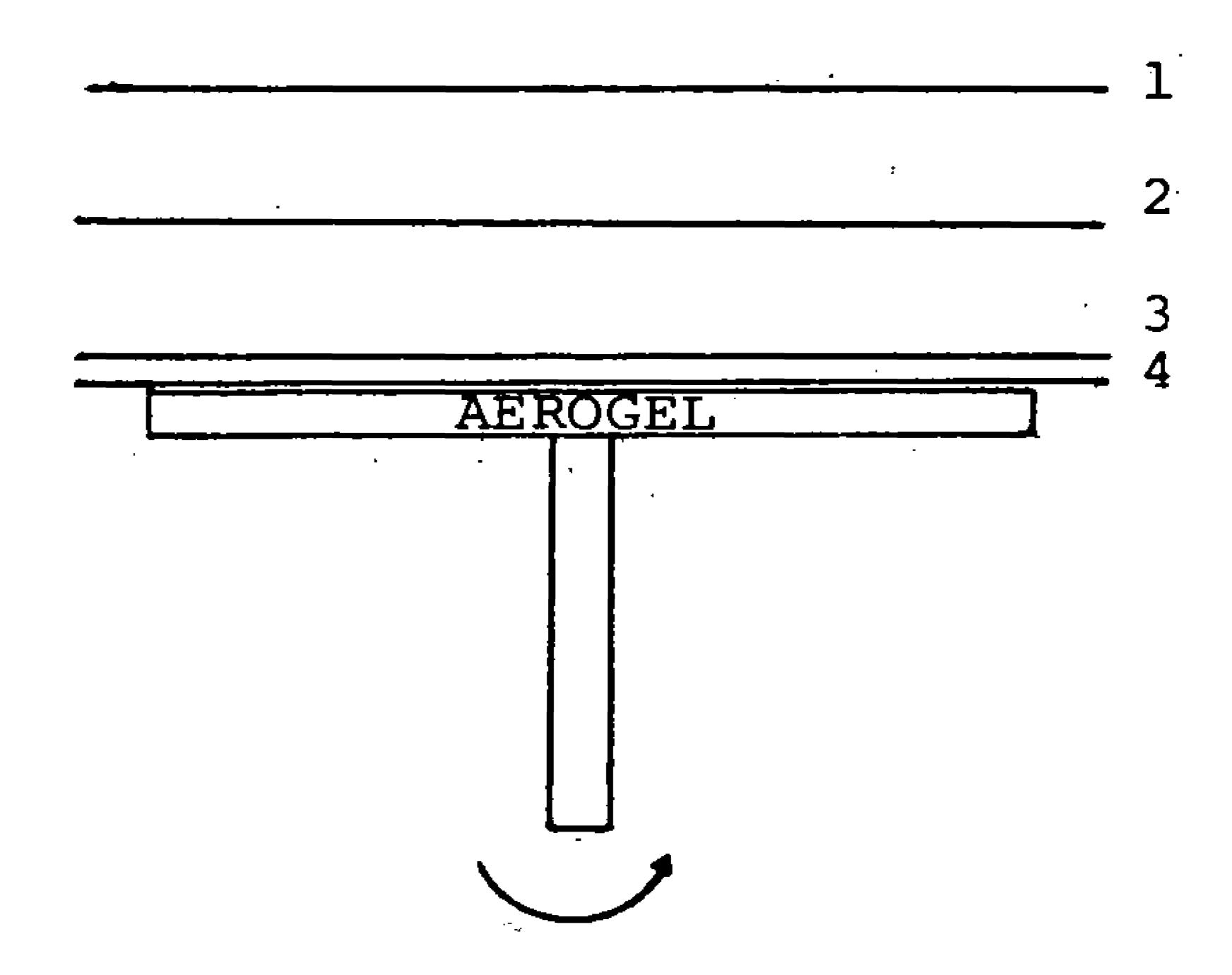
Figure 1. Schematic of the collector. 1, 2, 3 and 4 are polyester films. The aerogel plate is mounted on a rotating platform.
