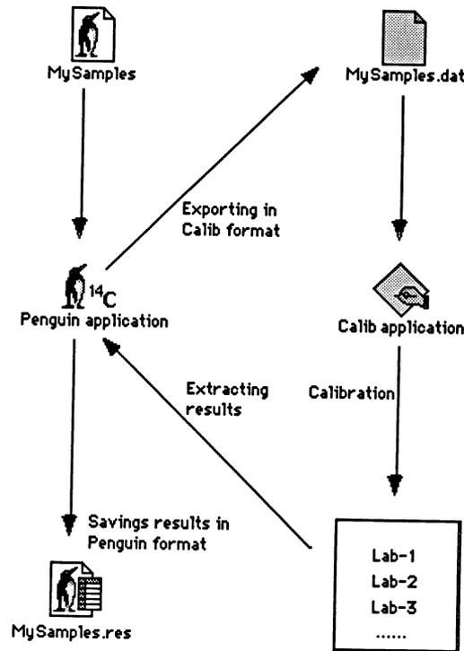
Fig. 1. Flowchart showing the role of *Penguin* in the calibration process. Data are kept in *Penguin* data files and CALIB input files are generated only when  $^{14}\text{C}$  dates need to be calibrated. *Penguin* then puts into a unique file the calibration results extracted from each output file created by CALIB.
