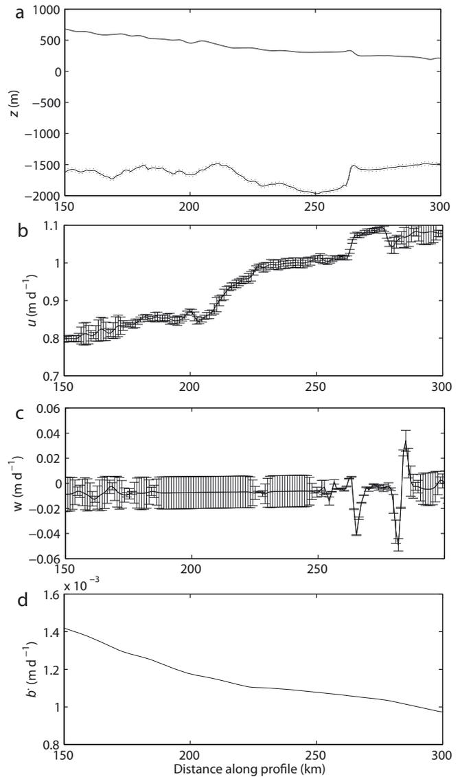
**Fig. 3.** The data and estimated data errors after interpolation onto the nodal points of the FE forward model. (a) Surface and bedrock topography with dots denoting the error range, (b) horizontal and (c) vertical surface velocities and corresponding error bars and (d) water equivalent accumulation rate.
