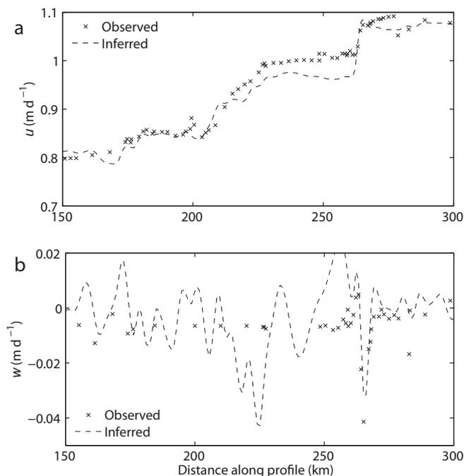
**Fig. 5.** Inversion experiment A: comparison between observed (crosses) and inferred (dashes) data along the flowline on Rutford Ice Stream. (a) Horizontal and (b) vertical velocity. The inferred surface data shown are the results of a forward step using the basal properties shown in Figure 4.
