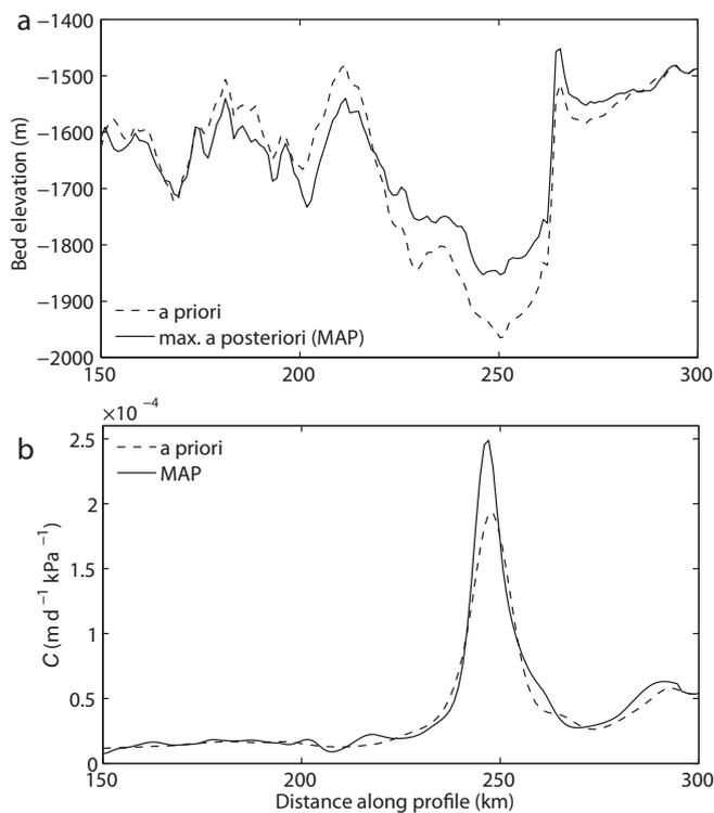
**Fig. 7.** Inversion experiment B: estimated (a) bedrock topography and (b) basal slipperiness distribution along the medial flowline of Rutford Ice Stream. The dashed curves correspond to (a) the prior bedrock distribution and (b) the prior basal lubrication distribution. The MAP solution is shown as a solid curve.
