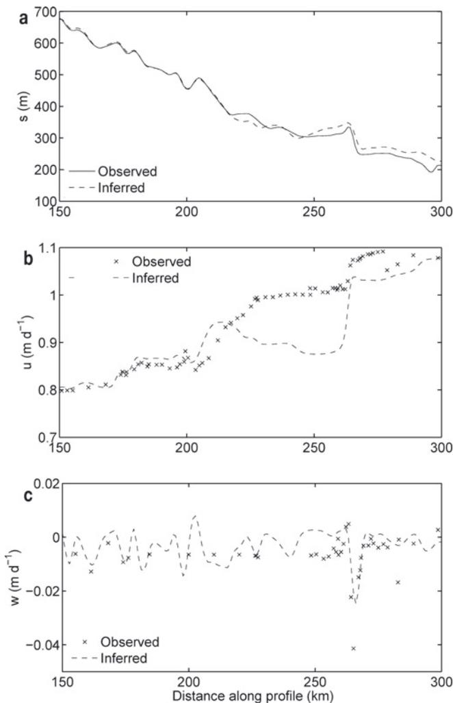
**Fig. 9.** Inversion experiment B: comparison between observed (solid curve in (a) and crosses in (b) and (c)) and inferred data (dashed curves) along the flowline on Rutford Ice Stream. (a) Surface topography, (b) horizontal and (c) vertical velocity. The inferred data correspond to the FE prediction for the MAP solution shown in Figure 7.
