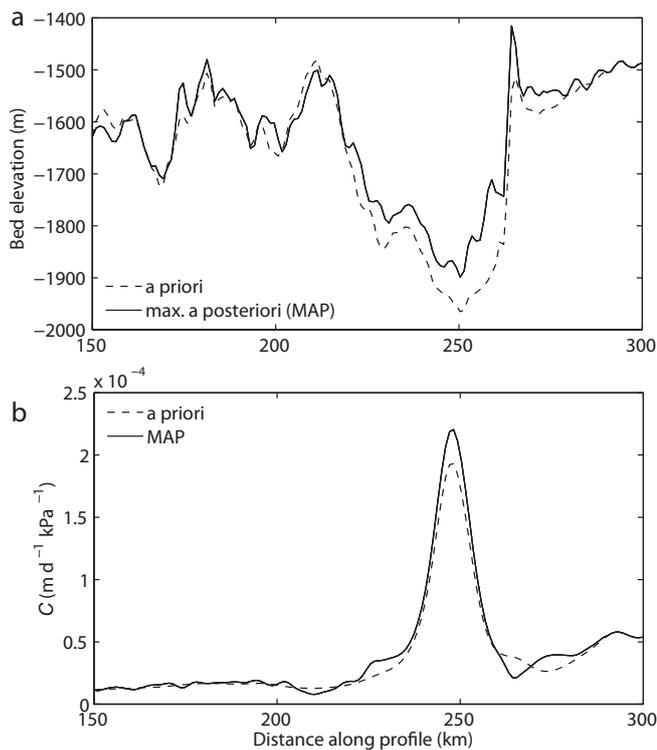
**Fig. 4.** Inversion experiment A. Solid curves show inferred (a) bedrock topography and (b) basal slipperiness distribution for the selected flowline on Rutford Ice Stream. The dashed curves show (a) the prior bedrock distribution obtained by interpolating the airborne radar data using BLUE to the forward FE grid and (b) the prior basal slipperiness distribution.
