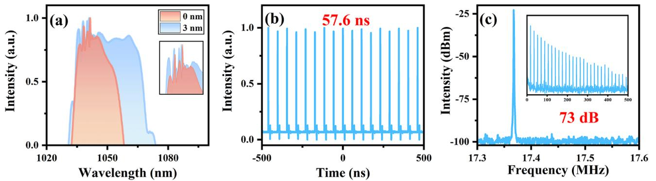
**Figure 2.** Experiment results. (a) Spectra: red is the mode-locked spectrum when the  $\Delta\lambda_f$  is 0 nm; blue is the mode-locked spectrum when the  $\Delta\lambda_f$  is 3 nm; inset shows the zoom-in of the CW state. (b) Pulse train. (c) RF spectrum.
