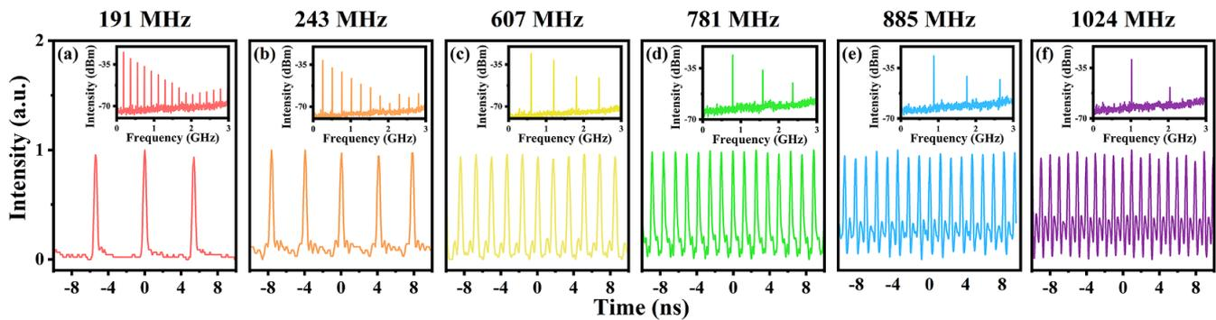
**Figure 4.** HML pulse train and RF spectrum: (a) 11th, (b) 14th, (c) 35th, (d) 45th, (e) 51st and (f) 59th harmonic orders.
