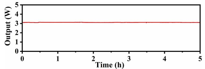
**Figure 7.** Power stability measurement of the mode-locked MO within 5 hours.
