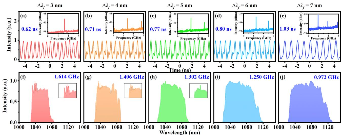
**Figure 5.** Experimental results under different  $\Delta\lambda_f$ . (a)–(e) Pulse train; inset, RF spectrum. (f)–(j) Spectra; inset, zoom-in of the CW state.
