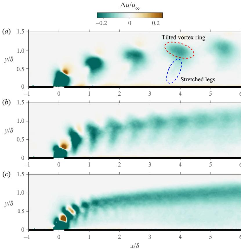
Figure 6. Plots of the boundary layer subtracted streamwise velocity field,  $\Delta u$ , normalised with the free-stream velocity when the jet is at peak blowing, i.e. at phase-locked value of  $\phi = 90^\circ$ , for (a) case 22, (b) case 23 and (c) case 24. These cases have the same aspect ratio and velocity ratio, resulting in the same momentum ratio per cycle of actuation, but differing actuation frequency.
