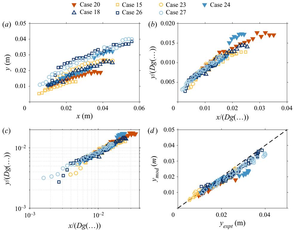
Figure 8. (a) Trajectories for all cases listed in table 1 which satisfy vortex interaction, in the near field. (b,c) The trajectories have been scaled by the corresponding  $g(\dots)$  as defined in (4.4) based on the respective coefficients in table 3. (d) Comparison of the time-averaged trajectories between the experimental data ( $y_{expt}$ ) and the newly derived model ( $y_{mod}$ ).
