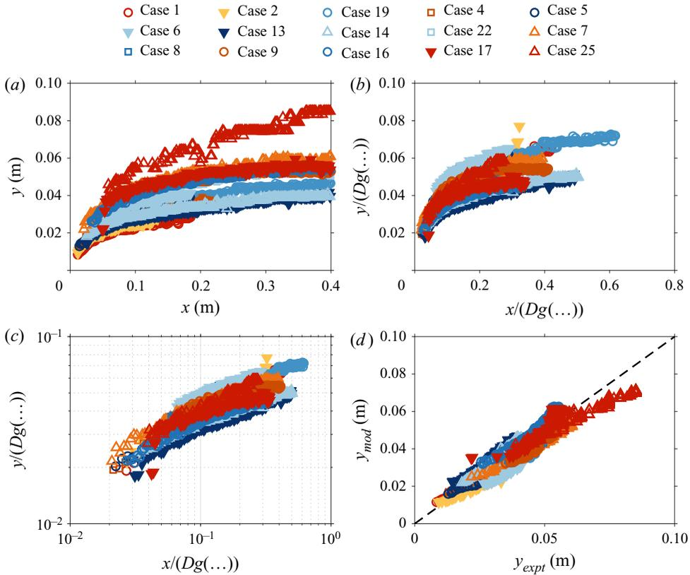
Figure 11. (a) Trajectories for all cases listed in table 1 where there is no vortex interaction in the far field. (b,c) The trajectories have been scaled by the corresponding  $g(\dots)$  as defined in (4.15) based on the respective coefficients in table 3. (d) Comparison of the time-averaged trajectories between the experimental data ( $y_{expt}$ ) and the newly derived model ( $y_{mod}$ ).
