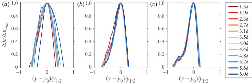
Figure 7. Self-similarity analysis for the cases presented in figure 6. (a)  $f = 100$  Hz, (b)  $f = 200$  Hz and (c)  $f = 400$  Hz. The velocity deficit  $\Delta u$ , following subtraction of the unperturbed flow field, is normalised by the maximum velocity-deficit value of the profile ( $\Delta u_{min}$ ) while  $y$ ,  $y_0$  and  $y_{1/2}$  represent the wall-normal location, wall-normal location at which the maximum velocity deficit occurs and the jet half-width, respectively.
