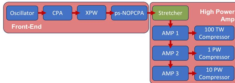
**Figure 1.** Schematic diagram of the ELI-NP HPLS. Marked with green is the stretcher that was updated during the activities reported here.
