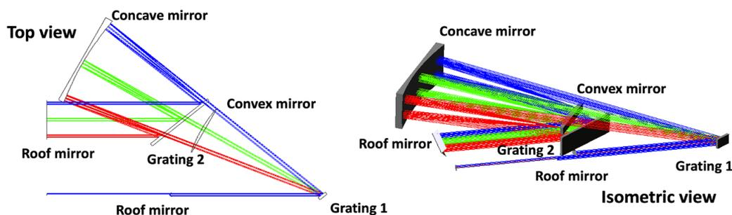
**Figure 2.** Schematic diagram of the Offner-type stretcher implemented at the ELI-NP HPLS.
