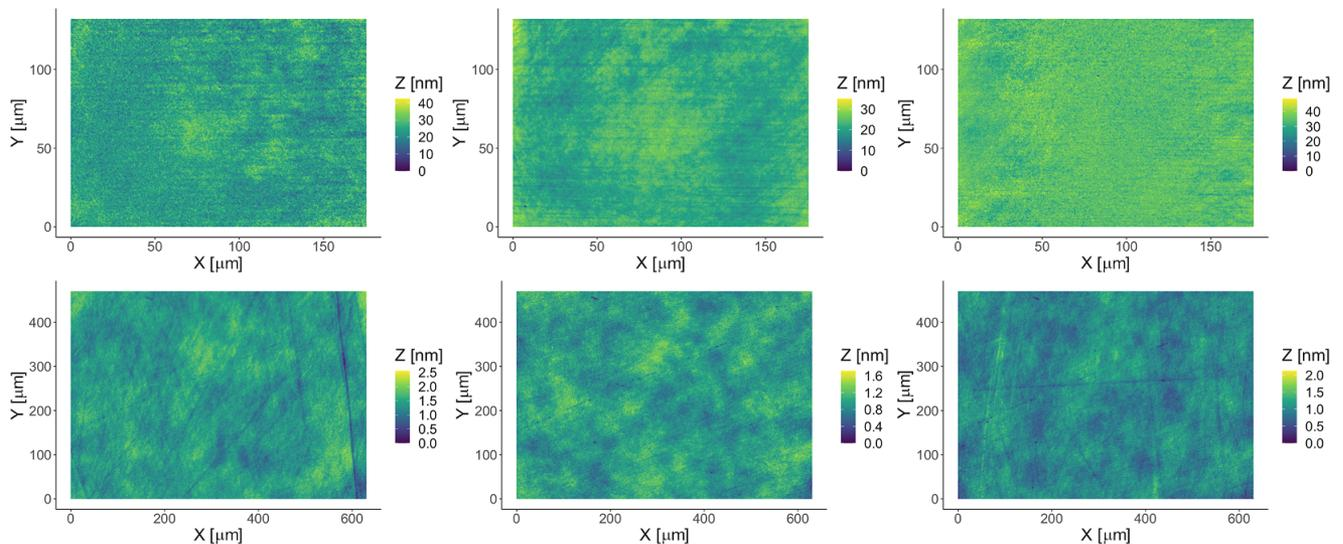
**Figure 3.** Roughness measurements for the old mirror (top row) and new, highly polished mirror (bottom row) performed on three separate locations.
