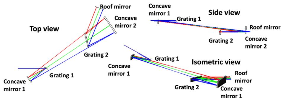
**Figure 4.** Schematic diagram of the new reflective Martinez-type stretcher implemented at the ELI-NP HPLS.
