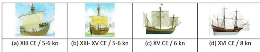
**Figure 4.** Ships. (a) Cinque Ports. (b) Cog. (c) Caravel. (d) Galleon (Batchelor and Chant, 2006).
