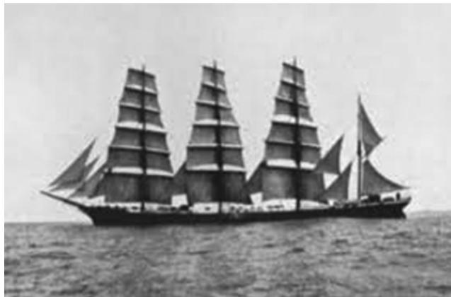
Figure 11. The Parama windjammer braced with fanning (Villers, 2009).
