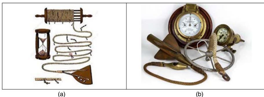
**Figure 1.** Logs. (a) Outboard log–chip log (2021). (b) Walker's mechanical log (paradeantiques.co.uk).
