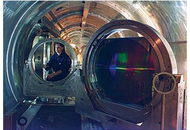
**Figure 1.** Inside the pulse compressor of the NOVA Petawatt – the first petawatt class laser worldwide (picture courtesy of LLNL).
