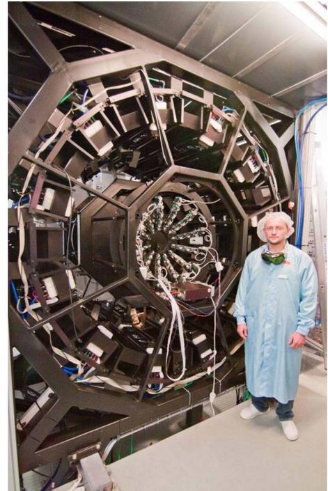
**Figure 12.** The final amplifier of POLARIS (picture courtesy of Helmholtz Institute).
