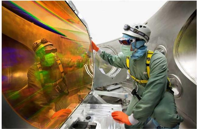
**Figure 3.** One of the Orion pulse compressor gratings (picture courtesy of AWE).
