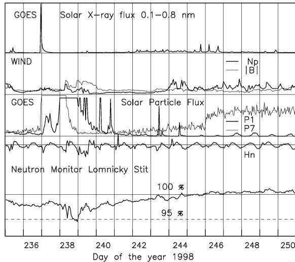
**Figure 2.** FD on the 238th day (26 August) in 1998: temporal evolution of NM measurements with a resolution of 1 hour (the bottom part of the y-axis), from top: solar X-ray flux (GOES), proton density  $n_p$  and interplanetary magnetic field intensity  $|B|$  (ACE), proton fluxes P1, P7 and magnetic field component  $H_n$  (GOES).
