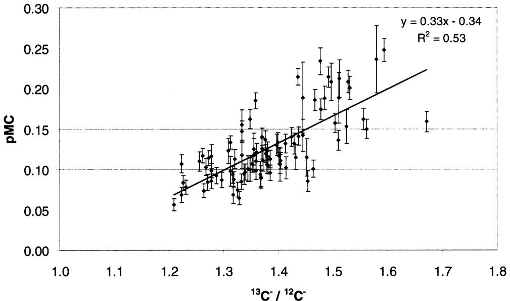
Figure 7 Correlation between the pMC values of targets graphitized from a large volume of  $\text{CO}_2$  made from IAEA C1 and their  $\text{CH}^-$  output.
