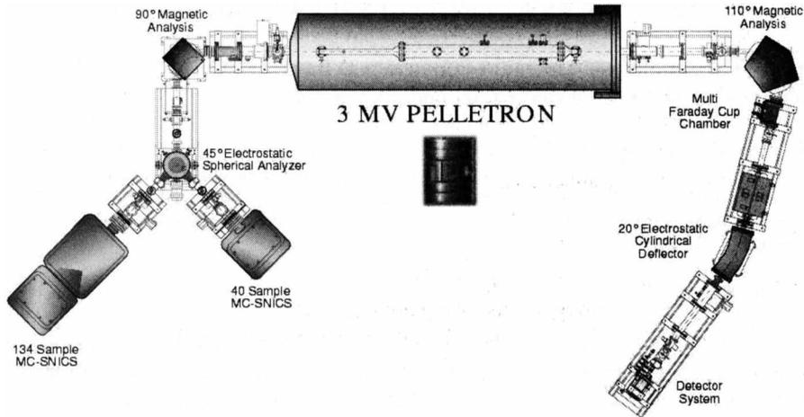
Figure 1 Artemis, 3MV Pelletron AMS system
