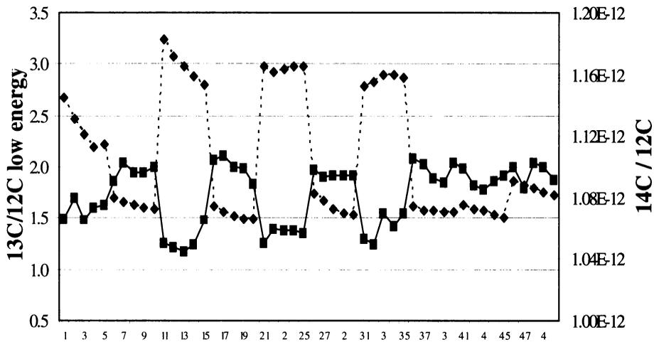
Figure 3 The  $^{14}\text{C}/^{12}\text{C}$  ratio (squares) is anticorrelated to the  $^{13}\text{C}^-/^{12}\text{C}^-$  ratio (diamonds), which reflects the  $\text{CH}^-$  output of the target.
