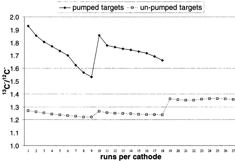
Figure 5 Variations of CH<sup>-</sup> output during the runs for pumped (diamonds) and unpumped (squares) targets.
