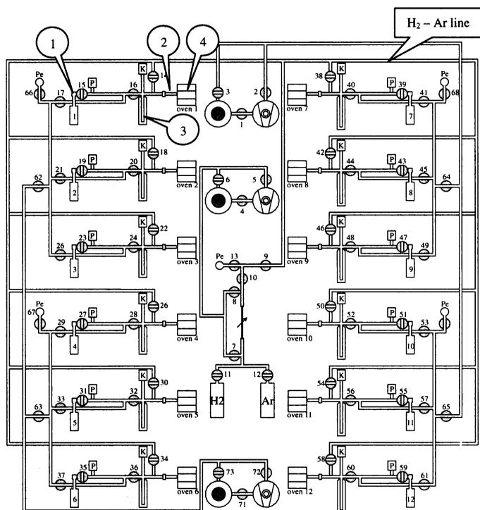
Figure 2 Schematics of the semi-automated graphitization system: 1 - vacuum line; 2 - reduction tube; 3 - cold finger (see text for details).
