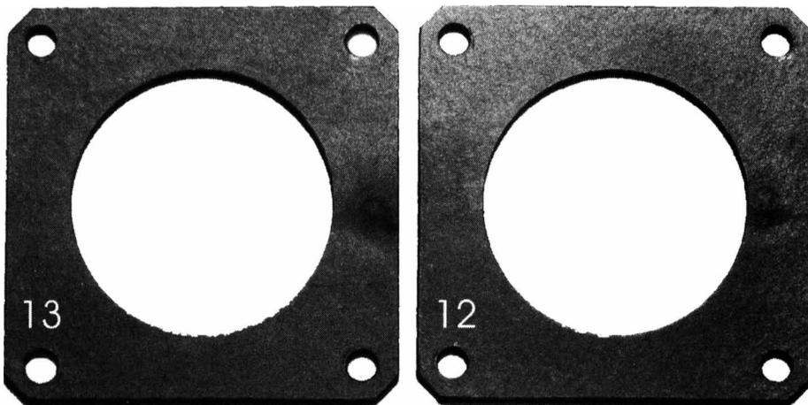
Figure 4 Diaphragms in front of the  $^{13}\text{C}^{3+}$  and the  $^{12}\text{C}^{3+}$  offset Faraday cups after the high-energy magnet showing the impact of the  $^{13}\text{C}^{3+}$  and  $^{12}\text{C}^{3+}$  beams coming from the corresponding  $\text{CH}^-$  molecules.
