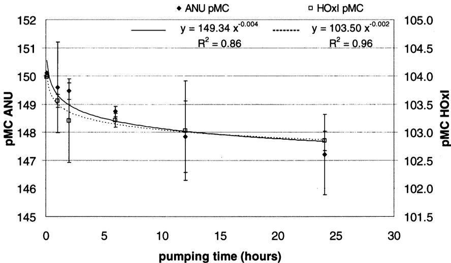
Figure 6 Average measured pMC decreases with the pumping time on the targets both for ANU (diamonds) and HOXI (squares) targets.
