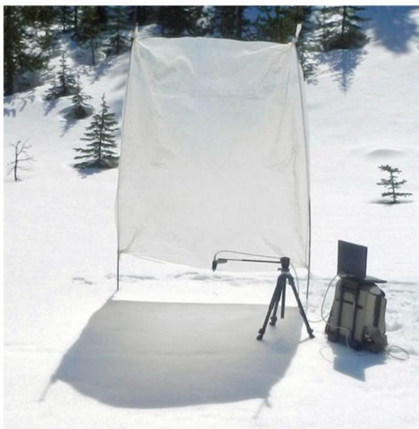
**Fig. 3.** Instrument setup for acquiring reflectance measurements with the field spectrometer.
