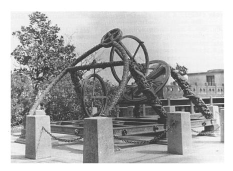
Abridged Armilla. At the beginning of the Yuan Dynasty, astronomer Guo Shou-jing simplified the complicated ancient instrument so as to separate the circles of the horizontal coordinate system from those of the equatorial system. It can avoid the obscuration of the observable sky region by the many rings of the old instrument. It was made in 1437, the second year of the Zheng-Tong Reign of the Ming Dynastry.
