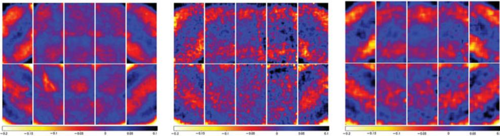
**Figure 2.** Distortion-correction maps, beyond third-order field terms, for SuprimeCam in 2002 (left), 2005 (middle) and 2012 (right). Corrections in the  $y$ -coordinate are shown, while those in  $x$  are generally similar. Units are pixels with a pixel scale of  $0.2''/\text{pix}$ .
