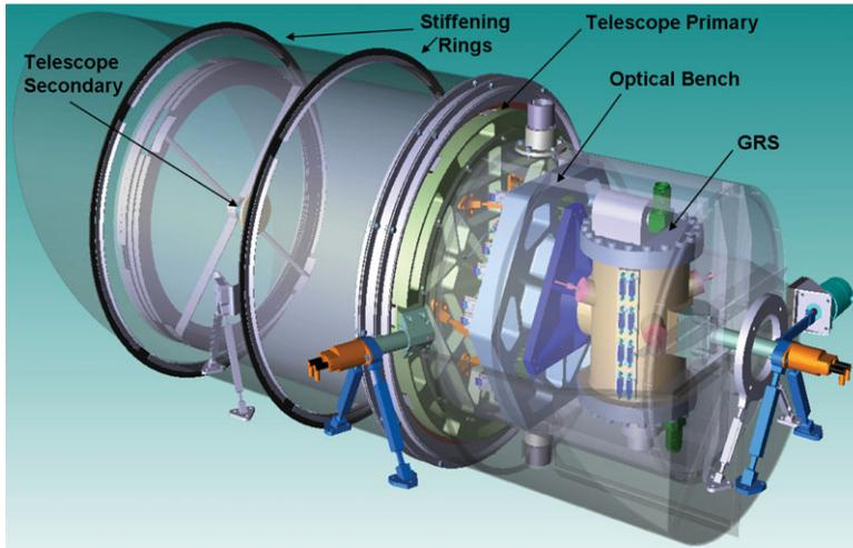
**Figure 2.** Optical assembly for LISA.
