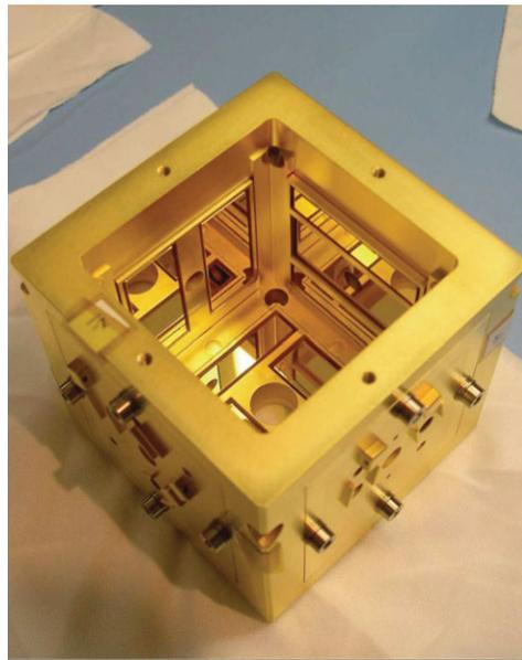
**Figure 5.** Electrode housing from Gravitational Reference Sensor designed for the LISA Pathfinder and LISA missions.
