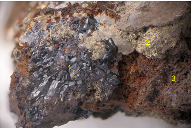
Figure 1. Theuerdankite (1) from the type locality associated with native silver (2) and chlorargyrite (3) in the cavity of strongly supergene-weathered material; Field of view: 3.6 mm; holotype specimen (P1P 59/2022); photo M. Gross.
