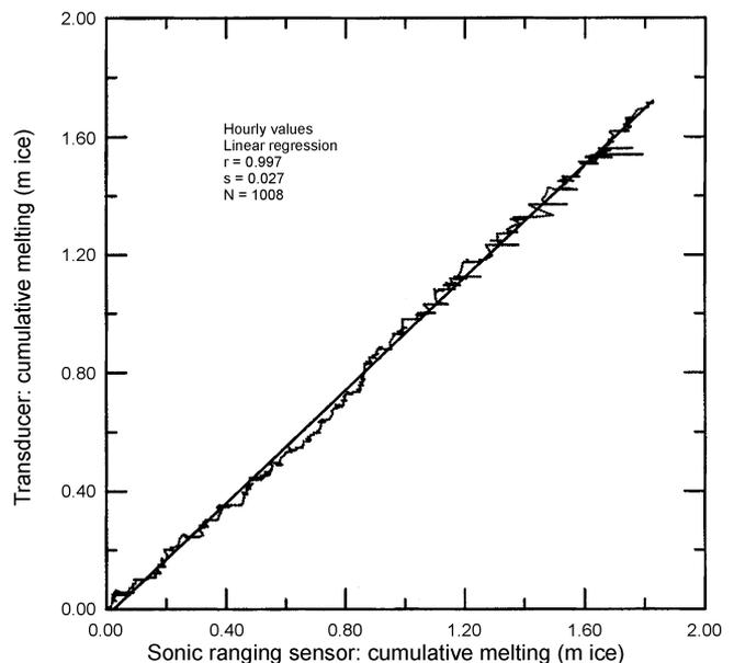
Fig. 2. The observed ablation using the pressure transducer plotted against SR50 observations.
