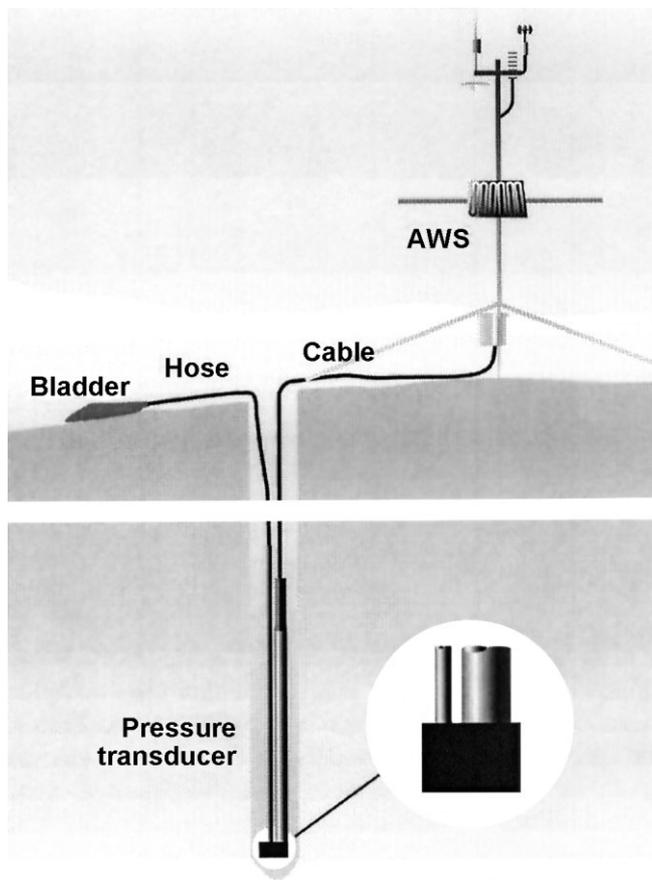
Fig. 1. Design and installation of the newly developed pressure transducer for automatic ablation observations.
