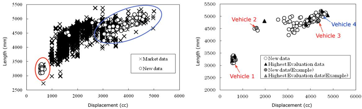
Figure 5. Relationship of displacement and length (new vehicle data and highest evaluation data).
